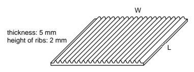
dimensions: 100 mm (W) x 100 mm (L) 150 mm (W) x 140 mm (L)
