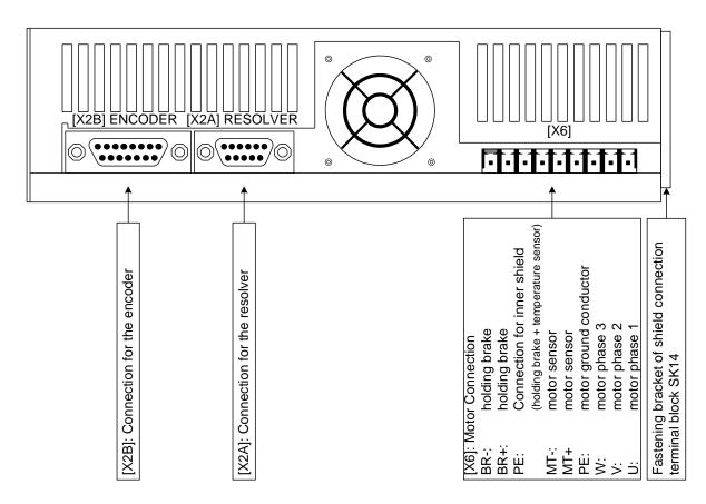
Figure 13: Servo positioning controller ARS 2102 FS: Bottom view
