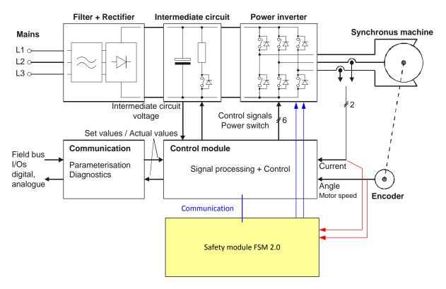
Figure 8: Schematic representation of the integrated safety technology (MOV)
