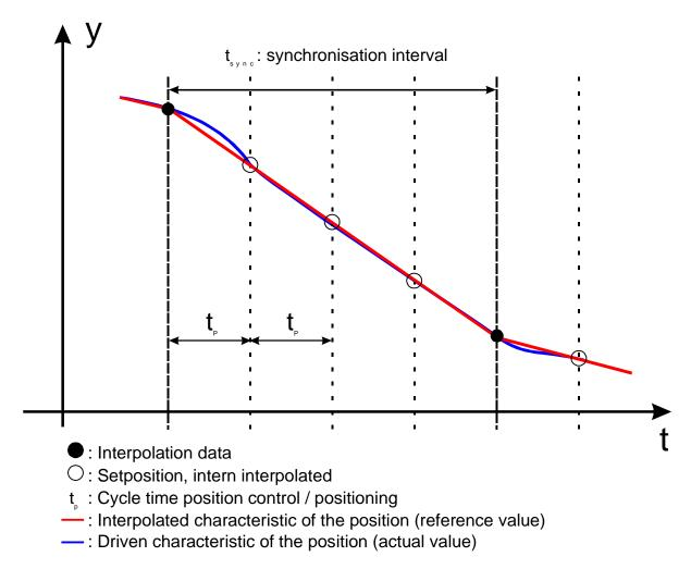
Figure 7: Linear interpolation between two data values
