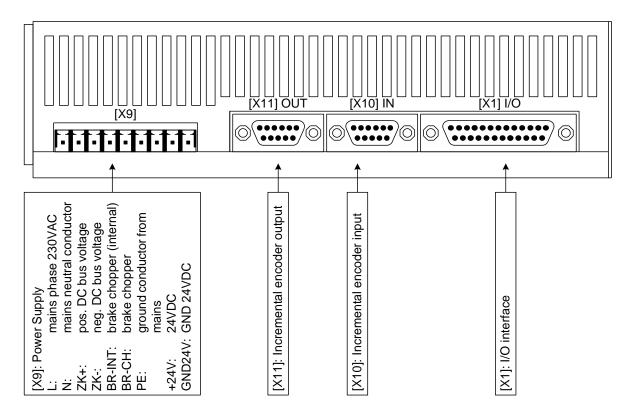
Figure 12: Servo positioning controller ARS 2102 FS: Top view
