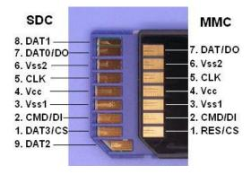
Figure 31: Pin assignment: SC/MMC card
