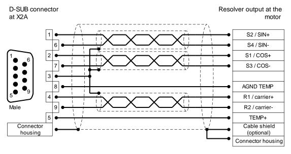
Figure 21: Pin assignment: Resolver connection [X2A]
