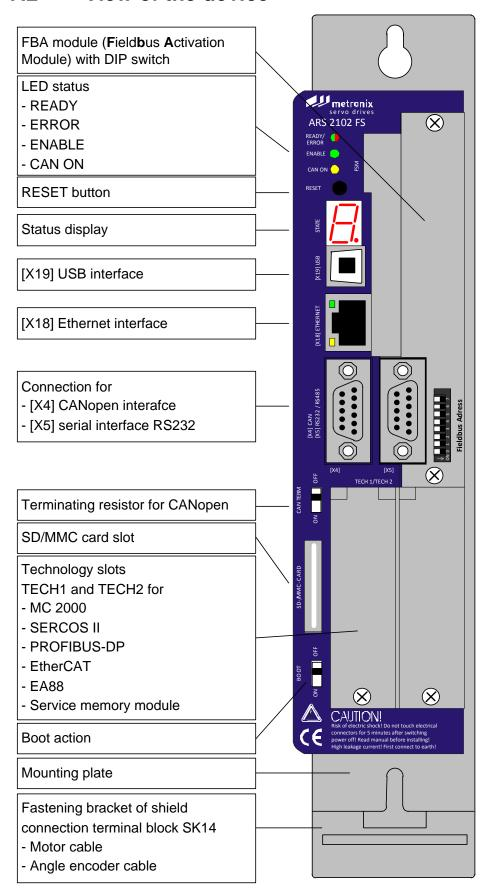
Figure 11: Servo positioning controller ARS 2102 FS: Front view
