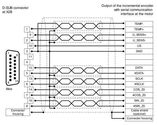
Figure 23: Pin assignment: Incremental encoder with serial communication interface (for example EnDat, HIPERFACE) – optional [X2B]
