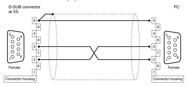
Figure 29: Pin assignment: RS232 null modem cable [X5]
