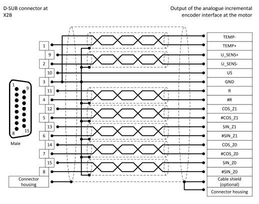
Figure 22: Pin assignment: Analog incremental encoder – optional [X2B]
