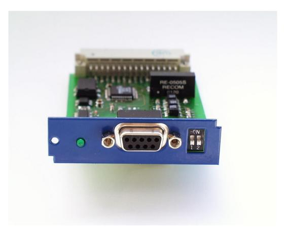
Figure 33: PROFIBUS-DP interface: Front view
