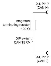
Figure 28: Integrated CAN terminating resistor
