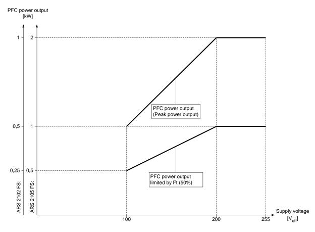
Figure 3: Performance curve of the PFC stage
