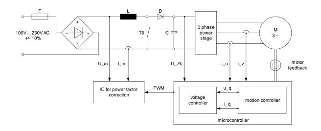
Figure 2: Schematic setup of PFC stage
