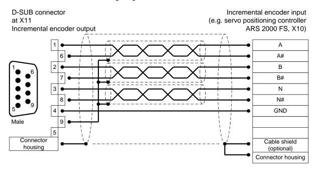
Figure 26: Pin assignment: Incremental encoder output [X11]
