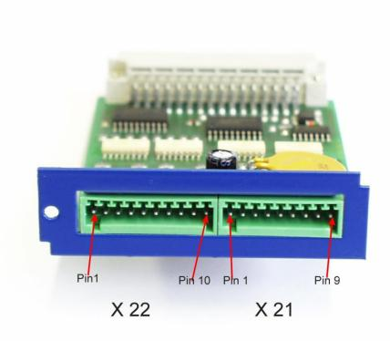
Figure 32: E88: Position of the pin-and-socket connectors [X21] and [X22] at the front plate
