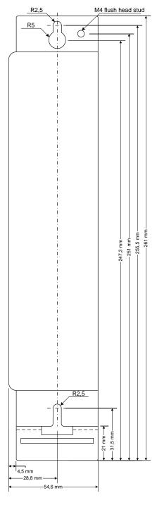
Figure 14: Servo positioning controller ARS 2100 FS: Mounting plate
