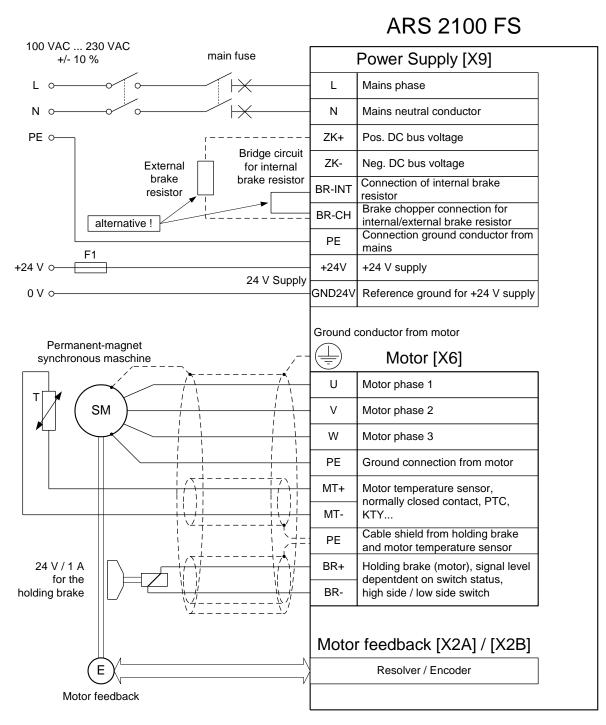
Figure 15: Connection to power supply and motor
