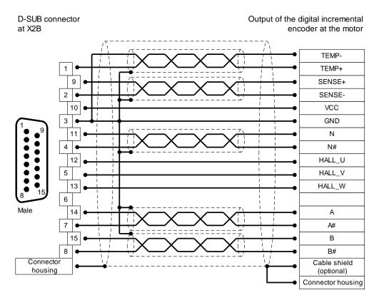
Figure 24: Pin assignment: Digital incremental encoder – optional [X2B]
