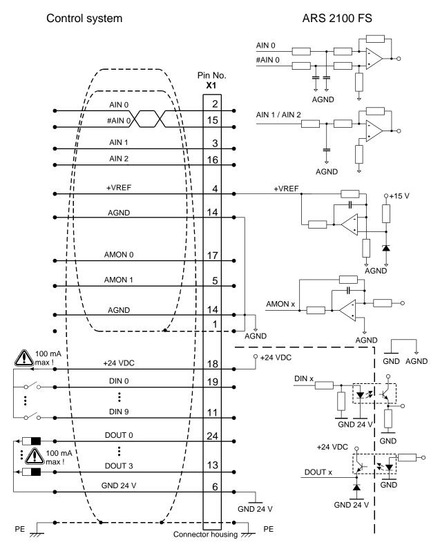
Figure 20: Basic circuit diagram connector [X1]
