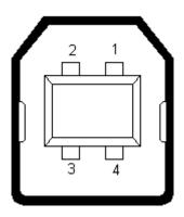
Figure 30: Pin assignment: USB interface [X19], front view
