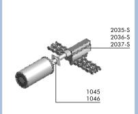
Chain lubrication with lateral connection
