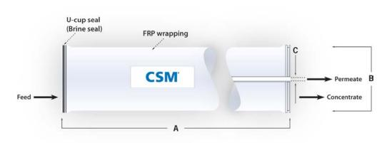
1. Each membrane element comes with one brine seal, one interconnector (coupler) and two o-rings. 2. All RE8040 elements fit nominal 8.0 inch (203 mm) I.D. pressure vessels.
