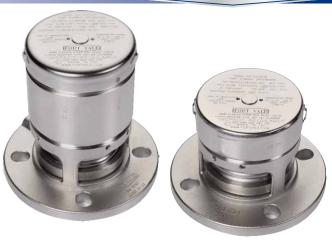
82.5mm Flanged Extended Hyper Maxi Pressure Only Relief Valve - Flange drilled 4 slots with a 145.0/152.4mm min/max PCD. (See below for drilling details) Suitable for a set pressure range of 75 to 204 PSI (5.17 to 14.07 Bar). Contact parts manufactured in 316 stainless steel. Fitted with Fortyt seals as standard.
