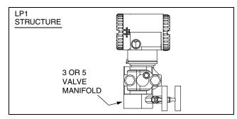
Figure 8. LP1 Shown Directly Mounted to Manifold
