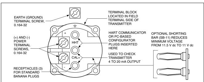
Figure 23. Field Terminal Block
