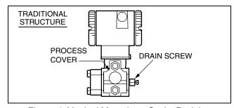
Figure 4. Vertical Mounting - Cavity Draining
