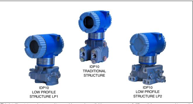
This Intelligent, two-wire transmitter provides precise, reliable, measurement of differential pressure, and transmits a 4 to 20 mA output signal with a superimposed HART digital signal for remote configuration and monitoring.
