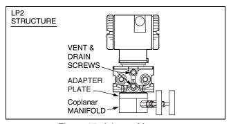
Figure 15. Adapter Mount to Existing Coplanar Manifold
