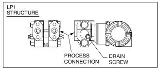
Figure 12. Horizontal Mounting with Drain Screw
