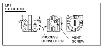
Figure 11. Horizontal Mounting with Vent Screw
