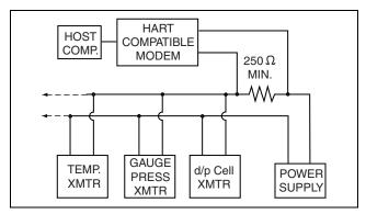
Figure 21. Typical Multidrop Block Diagram
