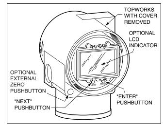
Figure 22. LCD Indicator with On-Board Pushbuttons
