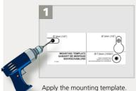
Apply the mounting template. Drill 1 hole for the cable. Drill 2 holes for the screws.
