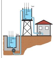
Two electrodes are used in this operation to control the tank level and another two for the well. One relay is used to activate the pump while the other for dry running / no
