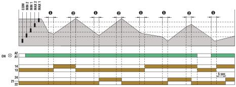
Filling tank and draining well function + alarm
