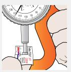
1.Tear off one section of the 2. Stick the tape on to the test 3. Using a micrometer such the thickness of the central pencil or similar rounded object portion of the tape replica and substract 50µm (2mils) from the reading. This result is the peak-to-valley profile height. Write the value on the tape.
