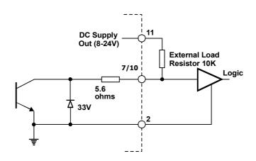
Driving a Logic Input such as a PLC or Electronic Counter
