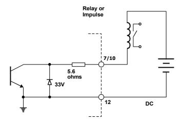
Driving an External Relay or Impulse Counter
