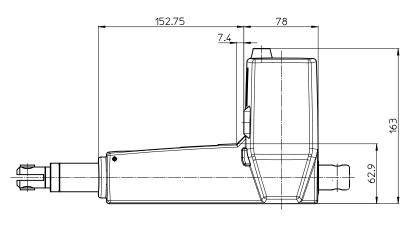
Standard installation dimensions with different combinations of Piston Rod Eyes and back fixtures to LA31.
