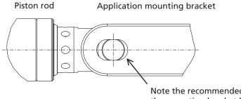
Note the recommended design for the mounting bracket hole
