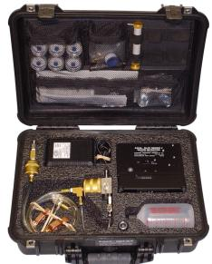
An outstanding feature of the Aqua-Glo<sup>®</sup> Kit is permanency of the fluorescing standard. Extreme care has been taken in perfecting a standard that will not deteriorate with age.
