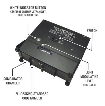
The Series V Aqua-Glo<sup>®</sup> was introduced in 2005 with an entirely new power supply. This power supply is external, automatically switching to work with either 120 VAC or 220 VAC, 50/60 Hz.
