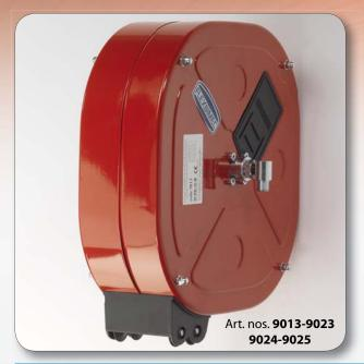
Automatic rewind, spring-driven hose reel, enclosed series, in painted steel, suitable for hoses of max 20 m length (ø hose 1/2") or max 25 m length (ø hose 3/8").
