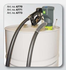
Diesel transfer kit, composed of electric 12 VDC, 24 VDC or 230 VAC pump, 3 m – cable with alligator clamps for battery connection (12 VDC and 24 VDC) or 2 m – cable with earth contact type plug, 1.6 m – suction hose with foot filter, 4 m – rubber delivery hose Ø 3/4" with anti-kink spring, hose tails and automatic dispensing nozzle with inlet swivel.
