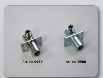
Interchangeable fluid shaft suitable for installation in hose reel series EVO in 1/2". They are available in galvanized and stainless steel AISI 304. In combination with the swivel joints of catalogue pages 224 and 225 they enable the use of a painted steel hose reel model also for fluids that require wetted parts in stainless steel (f. ex. water, AdBlue\*/DEF/AUS32), just by changing the components which are in contact with the fluid.
