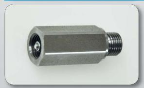
Parachute valve for lubricants pipeworks: blocks automatically the flow of lubricants inside of the pipework in case of leakages caused by failures or cracks of pipe components. Body in galvanized steel.
