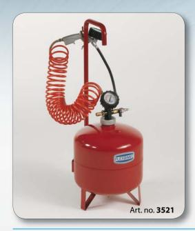
Portable, pneumatic tyre inflator with container of 16 I capacity, charging of compressed air manually, consisting of tyre inflating gun with pressure gauge (art. no. 7301) and 5 m – spiral hose.
