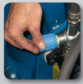
Pressure regulating valve for the control of the rewind strength.
