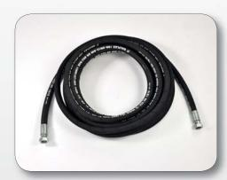
High pressure rubber hoses in accordance with SAE 100 R2AT, with swaged female BSP connection threads (swivel nuts), suitable for the supply of **grease** and **water** at high pressure. Internal structure in oil-resistant, synthetic rubber, coating in rubber highly resistant to abrasion, ozone
