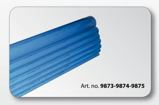
Calibrated pipes in extruded aluminium, in accordance with UNI 9006/1 and EN AW 6060 T6, suitable for the use with compressed air, water, inert gas or vacuum, with surface treatment in electrostatic painting in blue colour. Expansion coefficient: 0.024 mm/m°C).
