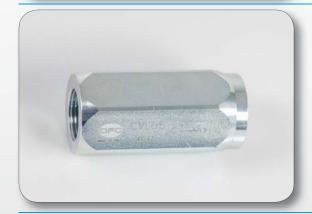
Non-return valve with high pressure gate valve, suitable for lubricants pipeworks. Body in galvanized steel, on demand also in stainless steel. Opening pressure 0.5 bar (on demand also 4 bar or 8 bar). Connections (BSP): inlet F – outlet F.
