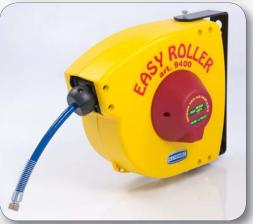
Automatic rewind, spring-driven hose reel, with plastic enclosure (made of nylon and polypropylene) and pivoting wall bracket, suitable for the use with compressed air and water (temperature range:  $-10^{\circ}$ C  $- +60^{\circ}$ C) and for hoses of 8 x 12 mm (or 10 x 14 mm) with a max. length of 15 m (or 10 m). Inlet connection air: 1/4'' BSP.
