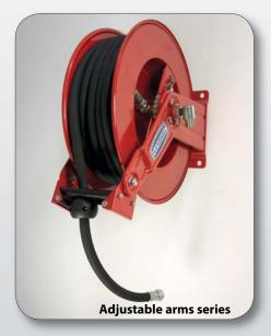
Automatic, spring – driven hose reel, adjustable arms series, in painted steel, including rubber hoses SAE 100 R1 AT with female connection threads, suitable for the supply of oil and antifreeze.
