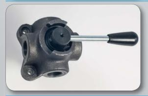
4-way flow diverter valve in cast iron, open center, with limited pressure drops. Made with 2 fixing holes  $\emptyset$  8.5 mm.
