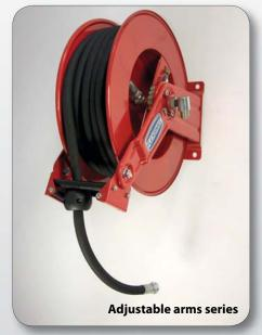
Automatic, spring – driven hose reel, adjustable arms series, in painted steel, including rubber hoses SAE 100 R2 AT with female connection threads, suitable for the supply of grease at high pressure. OPTIONAL: hydraulic spring braket kit for the controlled rewind of hoses Art. no. /HB.
