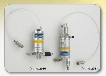
Automatic air separator devices, suitable to separate the air eventually present in the suction line from the oil, available with (= art. no. 2051) or without (= art. no. 2050) automatic pump stop system, **approved according to OIML R117-1**; includes also manometer for the control of the outlet pressure and non-return valve.
