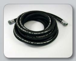
Low pressure rubber hoses in accordance with SAE 100 R6 – DIN EN 854, with swaged female BSP connection threads (swivel nuts), suitable for the supply of **diesel** and **petrol** at low pressure. Internal structure in oil-resistant, synthetic rubber, coating in rubber highly resistant to abrasion, ozone and atmospheric influences. Reinforcement: 1 textile braided and 1 steel wire braided layer.
