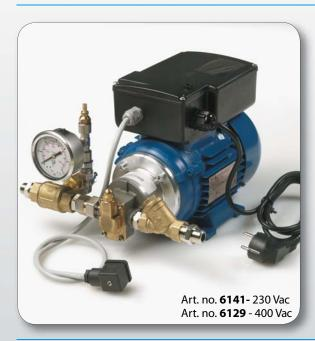
Electric, self-priming gear pump for the supply of oil, antifreeze, diesel, water at medium pressure; guarantees a constant flow and a low noise level. Pump body in stainless steel, gears in bronze and pump shaft in stainless steel.
