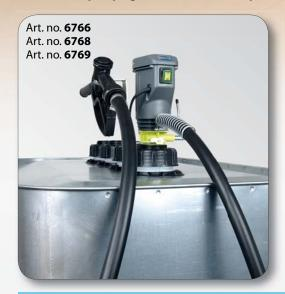
Diesel transfer kit, composed of electric 12 VDC, 24 VDC or 230 VAC pump, 3 m – cable with alligator clamps for battery connection (12 VDC and 24 VDC) or 2 m – cable with earth contact type plug (230 VAC), 1.6 m – suction hose with foot filter, 4 m – rubber delivery hose Ø 3/4" with anti-kink spring, hose tails and manual plastic nozzle.
