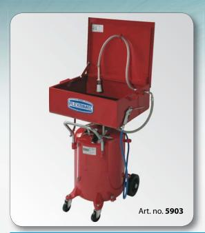
Mobile parts cleaner in painted steel, with closed circuit of detergent fluid, consisting of storage container with 65 l capacity with two wheels and two castors, cleaning basin with closable and removable cover, fluid-permeable cleaning brush which permits a continuous flow of the detergent and an accurate cleaning of parts, blow gun with rigid outlet. The system enables a continuous fluid circulation by pressurizing the container with compressed air at max. 0.5 bar.
