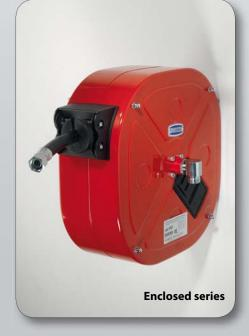
Automatic, spring – driven hose reel, enclosed series, in painted steel, including rubber hoses SAE 100 R2 AT with female connection threads, suitable for the supply of grease at high pressure. OPTIONAL: hydraulic spring braket kit for the controlled rewind of hoses Art. no. /HB.
