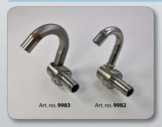
Low pressure swivel joints, suitable for hose reels in 1'1/4'' and 1'1/2'', with fixed fluid shaft and swivelling support, gooseneck assembly and hose tail connections Ø 33 mm and Ø 38 mm.
