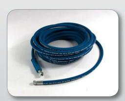
High pressure, **blue antistaining rubber hoses**, in accordance with SAE 100 R2AT, with swaged female BSP connection threads (swivel nuts), suitable for the supply of **water** at high pressure (f. ex. in combination with high pressure cleaners).
