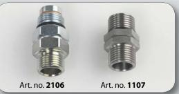
Art. no. **1107** Inlet swivel, in stainless steel AISI 304, connections 1/2" BSP (M), max static pressure 200 bar.
