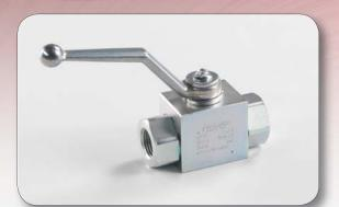
High pressure ball valve, with full port and lever handle, suitable for lubricants pipeworks. Body in galvanized steel. Connections (BSP): inlet F – outlet F.
