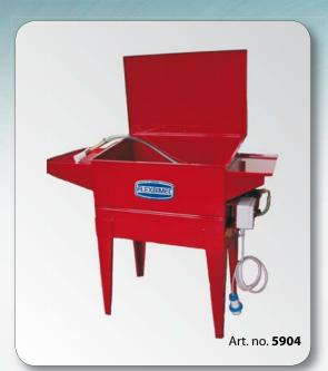
Stationary parts cleaner in painted steel, with closed circuit of detergent fluid, consisting of cleaning basin with 4 legs and closable and removable cover, hose with shower head, fluid-permeable cleaning brush which permits a continuous flow of the detergent and an accurate cleaning of parts. The system enables a continuous fluid circulation at 0.5 bar pressure by the use of an electric immersion pump.
