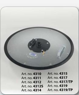
Follower plate with rubber edge, available in different dimensions to suit to the various types of grease drums. The follower plate causes a constant grease level inside of the drum and helps to avoid any air pockets inside of the grease close to the suction tube as well as any disposals of grease on the inner surface of the drum.
