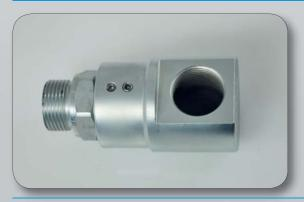
Swivel joint,  $90^{\circ}$  - type, with ball valve, self – lubricating. Body in galvanized steel, on demand also in stainless steel AISI 304. Connections (BSP): inlet F – outlet F.
