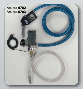
Electric, hybrid transfer pumps for diesel, fuel oil, bio-diesel (with suitable hoses), antifreeze (with or without water), suitable for the direct mounting on drums or tanks. These pumps are selfpriming, protection category IP 54, with ON-/OFF switch and an integrated connection thread BSP 2".
