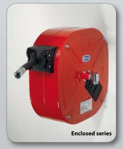
Automatic, spring – driven hose reel, enclosed series, in painted steel, including rubber hoses SAE 100 R1 AT with female connection threads, suitable for the supply of oil and antifreeze.
