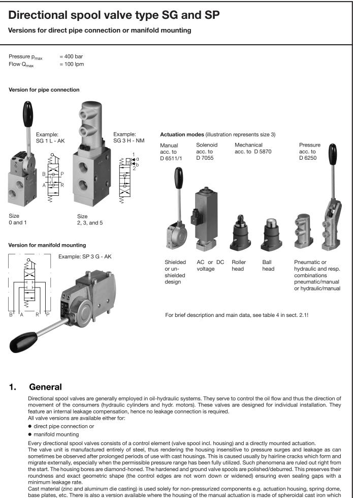
is intended especially for rough operation conditions or when these valves are connected in series.
