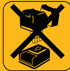
Do not charge damaged batteries
