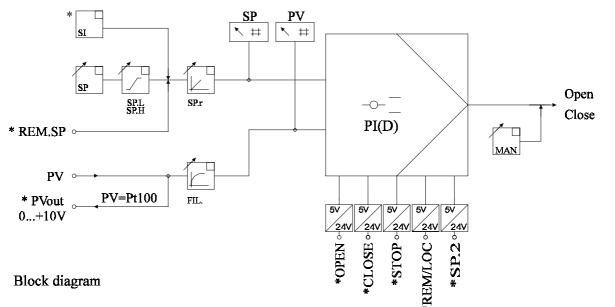
Setpoint limitation minimum value SP.L - setpoint low, maximum value SP.H - setpoint high. Only setpoints within the setpoint limits can be set by way of the keyboard.
