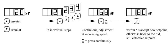
Setting range: SP.L to SP.H Locked setpoint input at SP.2 or REM. and S.C = 1
