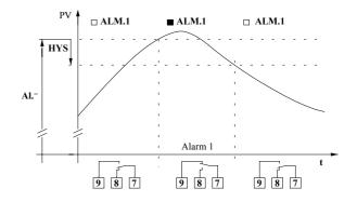
Alarm Type B for alarm relay 1
