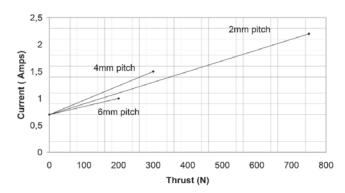
The above values are average values made with a stable power supply and an ambient temperature of 20° C.
