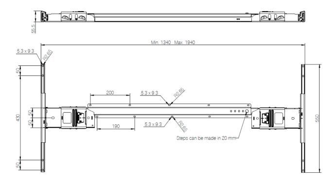
Figure 1 Kick & Click Adjustable dimensions in mm
