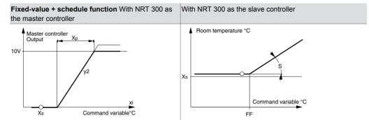
Output y2 or y1 of the master controller can influence multiple controllers. With setpoint adjustment knob X<sub>S</sub>, shift starting point FF can be selected, and with Pband X<sub>P</sub> the slope can be selected.
