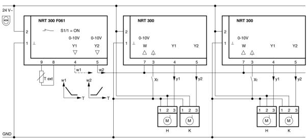
Outputs w1 (y<sub>1</sub>) and w2 (y<sub>2</sub>) (total load > 5 k $\Omega$ ) of the master controller to shift max. 10 × NRT 300
