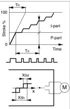
Open-Stop-Close signals (Proportional-integral control F041) In the case of an abrupt control offset, first a longer P pulse and then continuous smaller I pulses are output, until the control offset is smaller than half the switching range X<sub>Sh</sub>.
