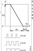
Pulse-Pause signals (proportional control F041) Control factor E (pulse duration/period duration) changes in proportion to the control offset. As a result, the average heating output also changes, as well as the stroke of a proportional thermal actuator such as a P-controller.
