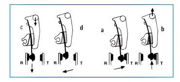
Furthermore, the elimination of return springs (a necessary part of the return mechanism in conventional relays) makes the relay remarkably resistant to impact.
