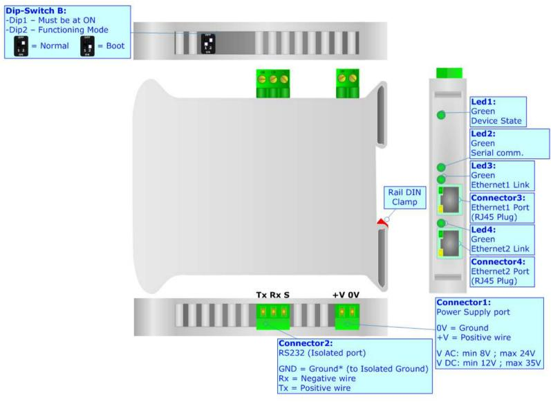
Figure 1a: Connection scheme for HD67591-232-A1
