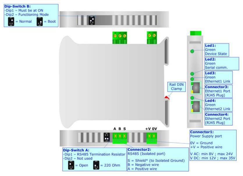
Figure 1b: Connection scheme for HD67591-485-A1
