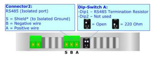
The maximum length of the cable should be 1200m (4000 feet).
