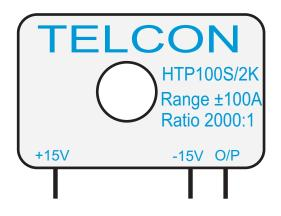
The HTP100S/2K is a closed loop Hall Effect Current Transformer suitable for measuring currents up to 100A. The product provides an output current into an external load resistance.
