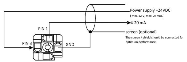
When replacing a 3-wire transmitter with a 2-wire transmitter NO changes to the wiring configurations are required.
