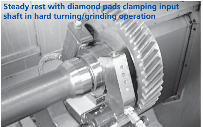
Steady rest clamping aircraft shaft
