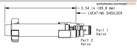
This FLeX Series, solenoid-operated 2-way, 2-position cartridge is a direct-acting directional poppet valve with a soft shift feature. Available in either normally open or normally closed configurations, these valves feature a pressure-balanced design, low leakage, and allow flow or blocking in both directions.
