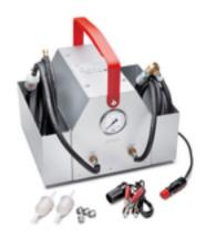
Electrical pump for ventilation of fuel systems of HDEP/MDEG diesel motors in utility vehicles. 24 V/DC power supply via battery terminals. Suction hose with integral fuel filter. Ventilation process can be precisely observed via an integrated pressure gauge with a measurement range of 0...10 bar, glycerine-filled. Automatic device switch-off at maximum pressure of 6.9 bar.
