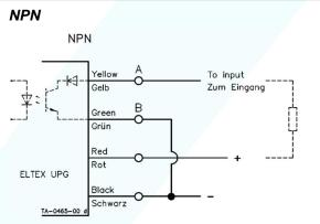
Configured as NPN open collector output (for input with pull-up resistor); low when yarn is not moving.
