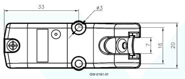
The UPG yarn break detector is fitted on the machine with two screws, maximum diameter 3 mm.
