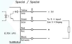
Configured as optocoupler output; high when yarn is not moving.
