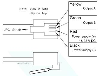
Output: Optocoupler, NC = normally closed Output load: max 10 mA, 35 V DC Max ON-STATE voltage drop: 2V DC at 10 mA
