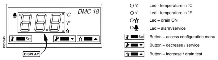
The DMC18 controls the alarms and the settings of the dryer operation and of the BEKOMAT drain.
