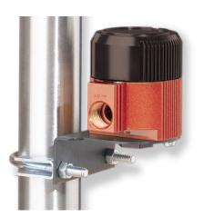
The durable PIH Pressure-to-Current Transmitter provides an economical solution for any process that requires a rugged instrument capable of interfacing a pneumatic device with a data acquisition/control system, controller, recorder, or other electronic instrument. This compact yet powerful unit accepts most pneumatic signals (3-15 psig, 0.2-1 bar, 3-27 psig, etc.) and accurately converts them to a proportional 4-20mA output.
