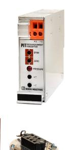
This rugged and reliable family of pressure-to-current transmitters provide an economical solution when a pneumatic device must interface with a data acquisition control system, controller, recorder, or other electronic instrument. Compact, yet powerful, these units accept a pneumatic signal (3-15 psig, 0.2-1 bar, 3-27 psig, etc.) and accurately convert it to a proportional 4-20mA (or 10-50mA) output.
