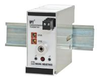
The high-performance IPT<sup>2</sup> Current-to-Pressure (I/P) DIN-style Transmitter converts a current signal to a pneumatic signal so that an electronic-based system such as a DCS, PLC, or PC can control a pneumatic actuator, valve, or damper drive. Available models accept a wide range of current inputs (4-20mA, 4-12mA, and 12-20mA) and provide a proportional pneumatic signal (3-15psig, 0.2-1 Bar, 20-100kPA, etc.).
