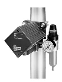
The rugged IPF Field-Mounted Current-to-Pressure Transmitter is designed specifically for installation in harsh environments. The two-wire IPF accepts a 4-20mA or 10-50mA input. It converts the input to a 3-15psig, 0.2-1bar, 15-3psig or 1-0.2bar pneumatic output signal, or to a wide variety of other commonly used pneumatic outputs and is available with an optional coalescing filter/regulator that combines both an air filter and a miniature supply line regulator.
