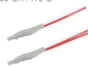
Platinum resistance temperature sensor on ceramic substrate protected by a heat-shrinkable sleeve and with PTFE isolated stranded wire. The TF101K version can be installed in motor or transformer windings. When build-in into windings do not pressure the sensor element. Precautions should be taken to protect sensor and extension leads against push and pull forces. Thermal response time  $T_{0,9}$  in the air 100 s, in water 19 s.
