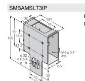
3073442 Protective housing with safety glas panel, for LT3 series
